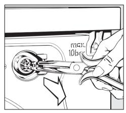
Use water pump pliers to withdraw the plastic filter by the bar (see illustration). Clean, put back and secure.
